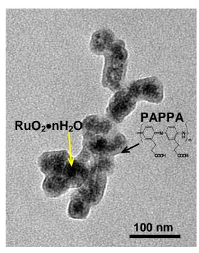
Figure 15. Transmission electron micrograph of nanocomposite of RuO<sub>2</sub> and the conducting polymer, PAPPA.<sup>9</sup>
