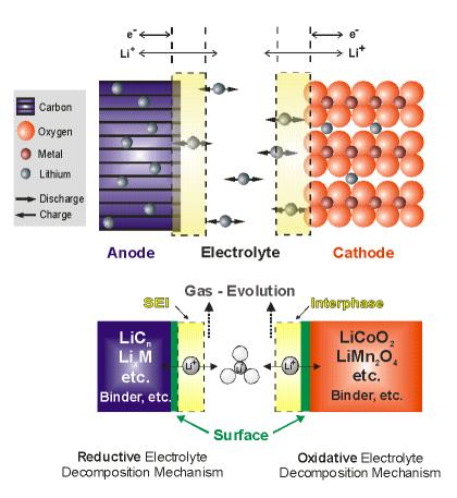
Figure 6. Operation principle, interphase formation, intra-electrode and intra-cell interfaces in lithium-ion cells.
