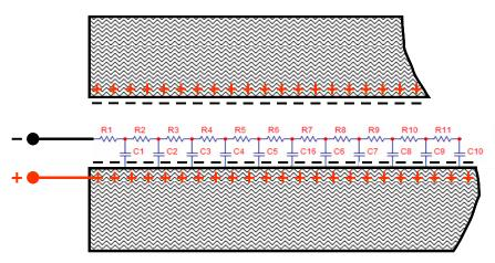
Fig. 16. Idealistic representation of a nanopore in a carbon electrode of an electrochemical capacitor.
