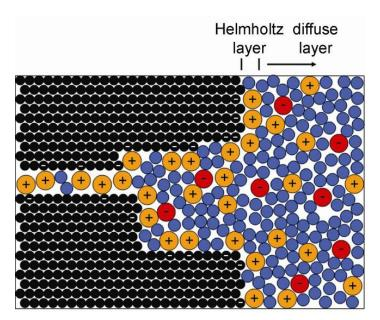
Figure 13. Schematic of how ion solvation may change in pores of different sizes during electric double layer charging (electrode material, black; solvent, blue; cation, orange, anion, red).
