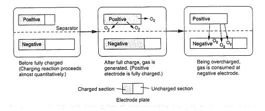
**Figure 10. Charge and overcharge processes for a sealed NiMH cell**. The different cell balance for NiMH results in a higher capacity for NiMH over Ni-Cd for the same size cell.
