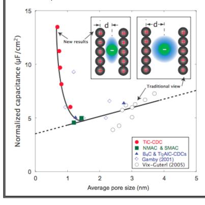
Dependence of material capacitance normalized by surface area on pore size. The results show that increasing the pore size above ~1 nm marginally increases the normalized capacitance. Decreasing the pore size below ~1 nm sharply increases the normalized capacitance due to constriction of the ion solvation shell (inset). Phenomena of this kind must be understood, described theoretically, and used in designing new material/solvent systems for capacitive energy storage.
