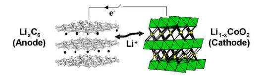
Fig. 11. A schematic illustration of a  $\text{Li}_x\text{C}_6/\text{Li}_{1-x}\text{CoO}_2$  lithium-ion cell. During discharge,  $\text{Li}^+$  ions migrate through the electrolyte and electrons flow through the external circuit, both moving from the anode (–electrode) to the cathode (+ electrode).
