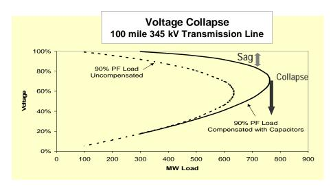
**Fig. 5.** The stable values of ac voltage when high levels of power are present in a **100-mile-long transmission line.** Note that as power flow reaches about 760 MW, a voltage collapse instability is encountered even with capacitor compensation. "PF" refers to the product of ac power and ac frequency and has units of joules.<sup>7</sup>
