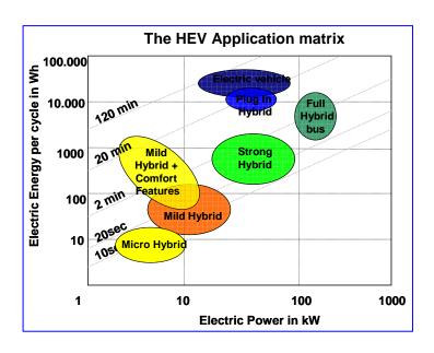
Fig 2. The total power and discharge power requirements for HEVs, including PHEVs and EVs. The deep discharge cycles required for PHEVs and EVs, combined with the requirements for long battery life, are not attainable with current technology.
