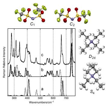
Figure 14. Calculated and scaled Raman spectra for (a)  $\operatorname{Et}_4N^+$   $\mathcal{D}_{2d}$  (solid line) and  $\mathcal{S}_4$  (dotted line), (b) TFSI transoid  $\mathcal{C}_2$  (solid line) and cisoid  $\mathcal{C}_1$  (dotted line) compared with (c) experimental Raman spectrum of  $\operatorname{Et}_4N$ TFSI recorded at 296 K.
