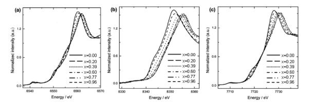
Figure B.1. Normalized Mn(a), Ni(b), and Co(c) K-edges XANES of  $Li_{1-x}Co_{1/3}Ni_{1/3}Mn_{1/3}O_2$  as a function of the amount of lithium in the lattice.<sup>2</sup>
