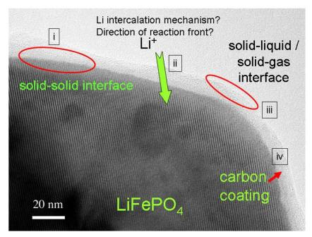
Figure 1. A battery system involves interactions among various states of matter. Transmission electron microscopy data courtesy of H. Gabsrisch.
