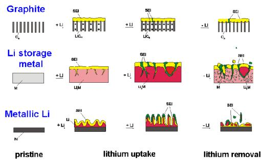
Figure 8. SEI stability and growth during continuous lithium uptake and removal for different anodes: graphite, lithium storage metals, and metallic lithium.
