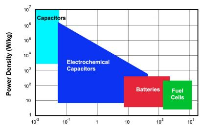
Figure 3. Power density as a function of energy density for various energy storage devices. <sup>2,1</sup>
