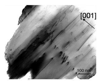
Figure 2. The large concentrations of dislocations in commercial LiCoO<sub>2</sub>, as revealed by transmission electron microscopy, raise fundamental questions with direct bearing on battery function. For example, what role do dislocations play in cycling performance? How do the dislocations change during cycling? What is their relationship to fracture formation/prevention?<sup>3</sup>
