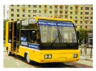
Fig. 20. Electric bus powered solely by an asymmetric electrochemical capacitor system. (Photo courtesy of ESMA Joint Stock Company)
