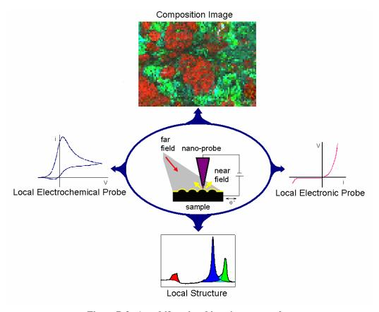
Figure B.3. A multifunctional imaging nanoprobe.
