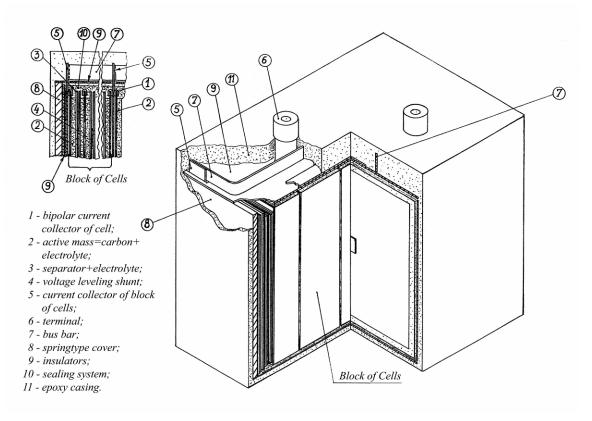
Fig. 17. Cutaway drawing of a bipolar symmetric electrochemical capacitor module. (Drawing courtesy of ELIT Company)
