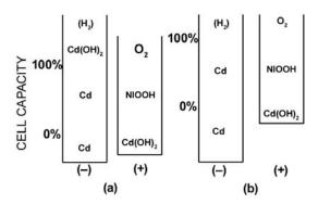
Fig. 9. Cell balance for (a) sealed and (b) vented Ni-Cd cells. In sealed cells it is essential to prevent  $H_2$  evolution on charge and essential that only  $O_2$  be evolved. The oxygen evolved from the nickel electrode diffused to the Cd electrode, where it reacts to form cadmium metal.
