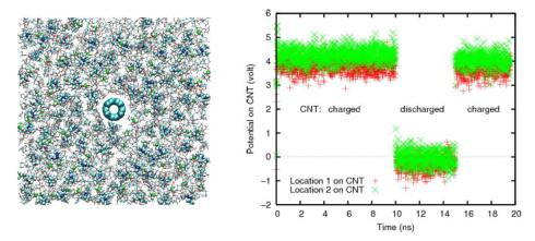
Figure 19. Molecular-dynamics simulations of an EC consisting of a periodic carbon nanotube forest in a common organic electrolyte (1 M TEA + BF4- in propylene carbonate). (Left) Initial molecular configuration. (Right) Time series of the carbon nanotube potential in response to a sudden change in surface charge, showing picosecond response. (Provided by L. Yang, B. Fishbine, and L. R. Pratt, unpublished, 2007.)
