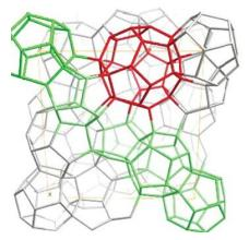
**Figure 11. Cagey structures.** Zeotype architecture of MIL-101 showing mesoporous cages with diameters of 29 Å (green) and 34 Å (red) featuring 12 Å pentagonal and 15 Å hexagonal openings.<sup>3</sup>
