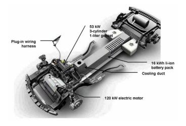
**Fig. 1. Phantom view of the recently announced GM Volt PHEV.** It shows the packaging of a small 3-cylinder engine and 53-kW engine-generator along with a 120-kW (EV1) traction drive and 16-kWh lithium-ion battery pack sourced from Cobasys-A123 Systems and Johnson Controls-Saft Advanced Power Solutions, LLC.
