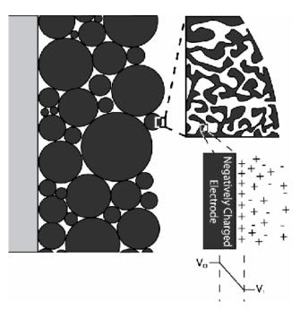
Figure 10. Schematic of an activated carbon-based EDLC illustrating the heterogeneity of particle size, pore size, and pore structure of the electrode that ultimately leads to performance limitations.
