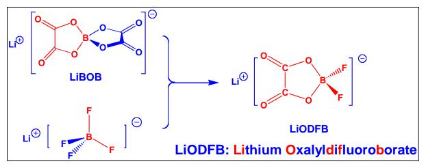
Figure 9. LiODFOB: a hybrid electrolyte salt material formed from LiBF<sub>4</sub> and LiBOB.
