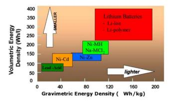
Fig. 7. Performance of several classes of batteries.
