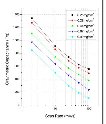
specific capacitance of 550 F/g at 100 mV/s and 190 F/g at a scan rate of 2 V/s (see figure).<sup>5</sup> XPS and HRTEM analysis indicate the reversible oxidation and reduction of vanadium (II–IV) arises from a monolayer surface film of an amorphous oxide/oxynitride. The exact mechanism, interaction with the aqueous KOH electrolyte, and the electrochemical stability are still unknown. These and other novel pseudocapacitance materials hold exciting promise for future generations of EES devices.
