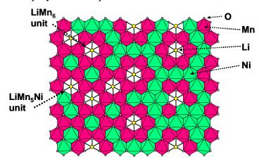
Figure 4. Schematic illustration of the cation arrangement in a layered, composite  $xLi_2MnO_3 \bullet (1-x)LiMn_{0.5}Ni_{0.5}O_2$  electrode structure in which  $LiMn_6$  units, characteristic of the  $Li_2MnO_3$  component (and disordered  $LiMn_5Ni$  units), are embedded as stabilizers in the residual  $LiMn_{0.5}Ni_{0.5}O_2$  component.<sup>8</sup>
