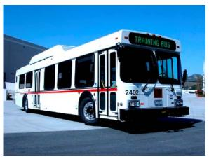
Fig. 21. Gasoline/electric hybrid bus with an electrochemical capacitor energy storage system. (Photo courtesy of ISE Corporation)
